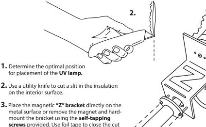
4. Use plastic **quick-nuts** to attach the **UV lamp** to the **"Z" bracket** as shown.
